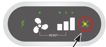
Flashing LED: maintenance required
